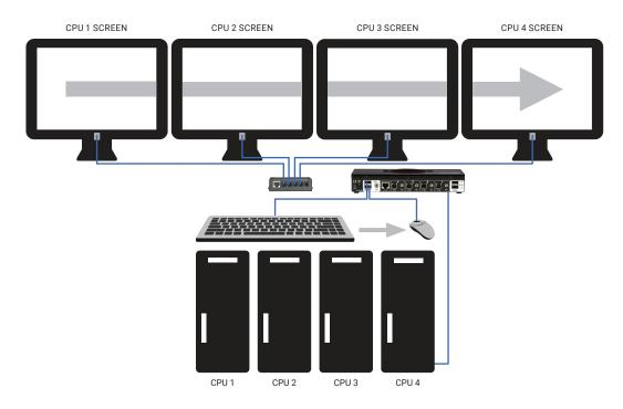
Glide and Switch Setup Using a Freedom II 4-Port Switch and LED Monitor Identification Kit
